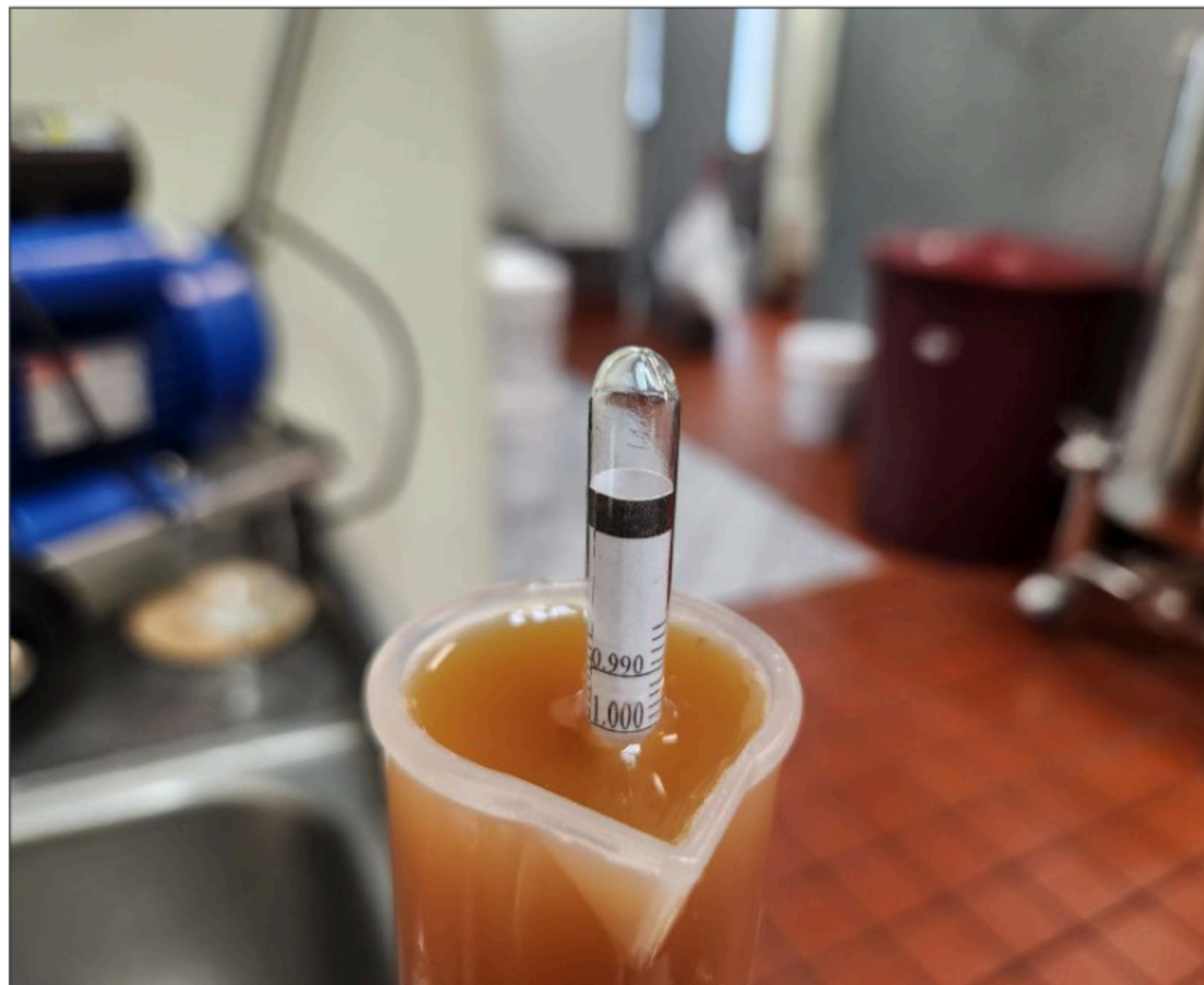
A hydrometer showing the apple raisin mead is finished fermenting. Courtesy Zydeco Meadery
